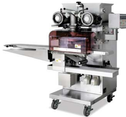
RHEON KN-135 ENCRUSTING MACHINE 20-100 Pc/min, 280 kg/hr extrusion For Filled Products, Suitable for soft & hard dough. Not suitable for fermented dough.
