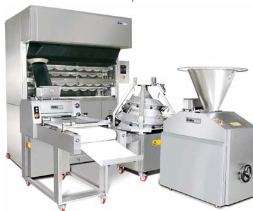
BREAD/RUSK PRODUCTION MAKEUP LINE Capacity: BREAD - Upto - 2400/hr Capacity: RUSK - 500 - 700 kg/hr
