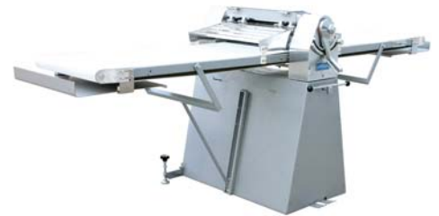
Heavy Duty Sheeter Model SM 630 with Oil Gear Box For Continues Production
