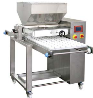
FORMEX TRAY TYPE CUPCAKE DEPOSITOR 1. Automatic Cupcake / Bar Cake Depositor 2. Automatic Injecting Machine for Cream/Jam 5-7 Nozzles for depositing choco-chips or Tutti Frutti Range: 5-65 cc batter upto 5000 pc/hr
